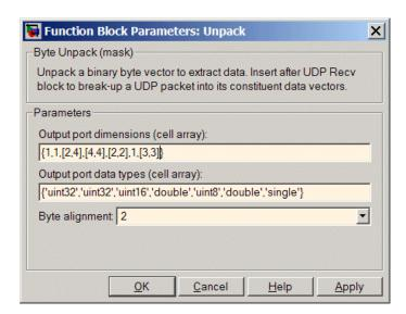
In addition, the **Byte alignment** setting matches as well. **Output port dimensions (cell array)** now includes scalar values and matrices to demonstrate entering nonscalar values. The example for the Byte Pack block assumed only scalar inputs.
