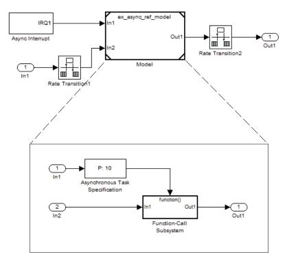
The Asynchronous Task Specification block must immediately follow the Inport block. Also, no branch can emanate from the signal connecting the Inport block to the Asynchronous Task Specification block.
