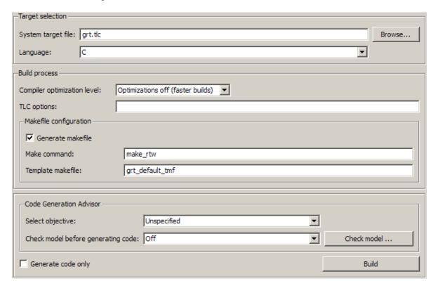
When the Simulink Coder product is installed on your system and you select an ERT-based target, the Code Generation General pane includes the following parameters. ERT-based target parameters require an Embedded Coder license when generating code.
