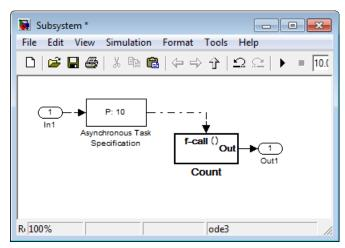
Whereas, if the priority of the Asynchronous Task Specification block is set to the empty matrix, [], then the Async Interrupt can have any value.
