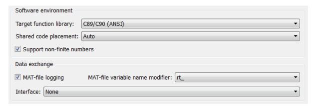
The Code Generation Interface pane includes the following parameters when the Simulink Coder product is installed on your system and you select an ERT-based target. ERT-based target parameters require an Embedded Coder license when generating code.
