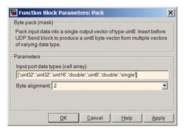
In the cell array, you provide the order in which the block expects to receive data—uint32, uint32, uint16, double, uint8, double, and single. With this information, the block automatically provides the proper number of input ports.
