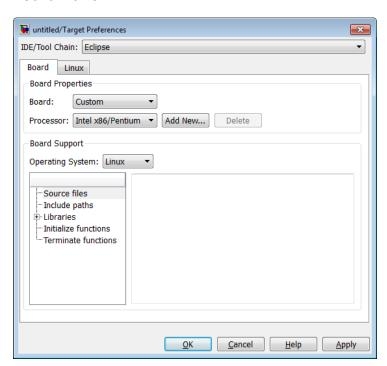
The following options appear on the **Board** pane, which has separate panels for **Board Properties**, **Board Support**, and **IDE Support** labels.
